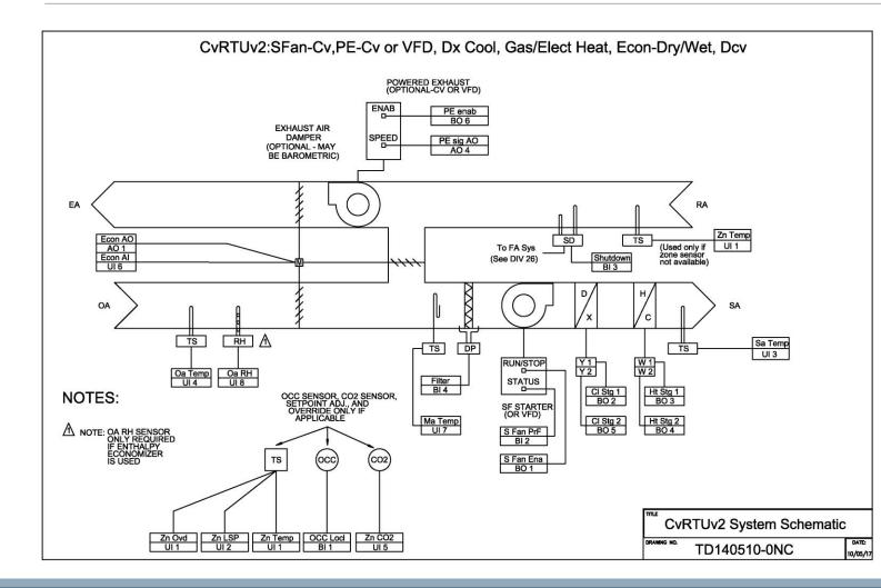
System schematic provided for each version in dxf format for editing. Physical point designators and BACnet names are shown on the schematic.
