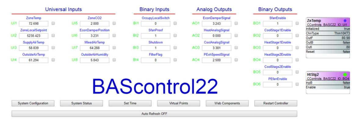
A common web browser is all that is needed to connect to the controller for configuration. Data points can be continuously refreshed. From this page you can launch into other pages.
