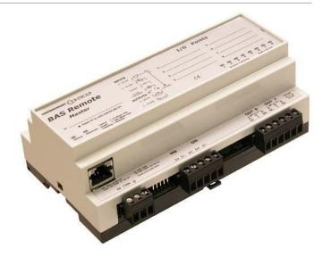
Contemporary Controls' BASremote was one of the first devices to be certified by Tridium as **Powered by Sedona Framework**.
