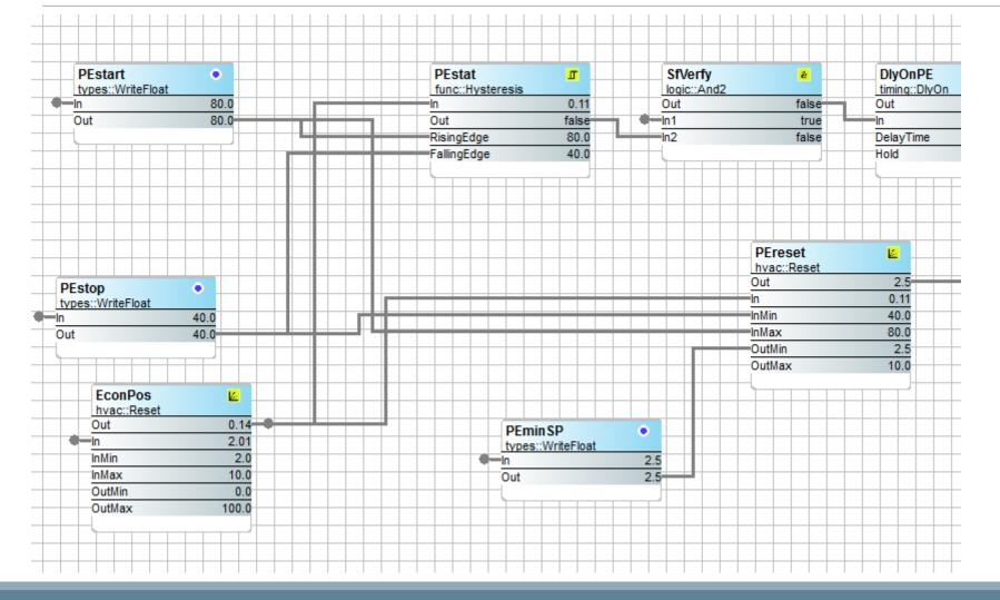
Using a drag-and-drop methodology, Sedona components are placed onto a wire sheet, configured, and linked together to create an application. Once placed on the wire sheet, components immediately begin execution thereby allowing for application debugging in real-time.
